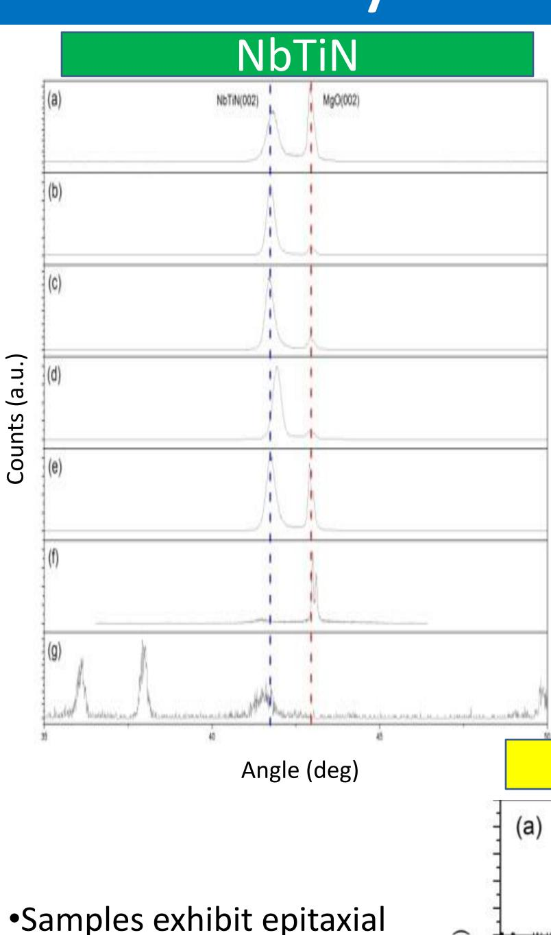
growth of the NbN layer with the MgO(001) substrate in the nominal, delta, superconducting structure even with two interlayers
