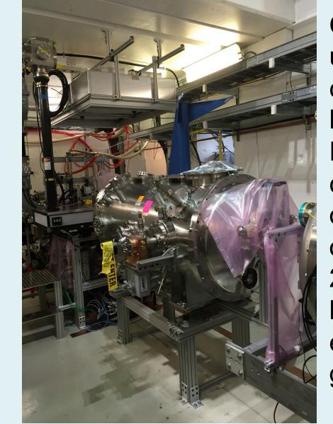
Capture Cavity 1 (CC1) upgrade work is now completed. The cryomodule has been installed on the FAST beam line. CC1 recommissioning and operation is expected to occur in late 2015/early 2016. Based on cavity horizontal tests it is
