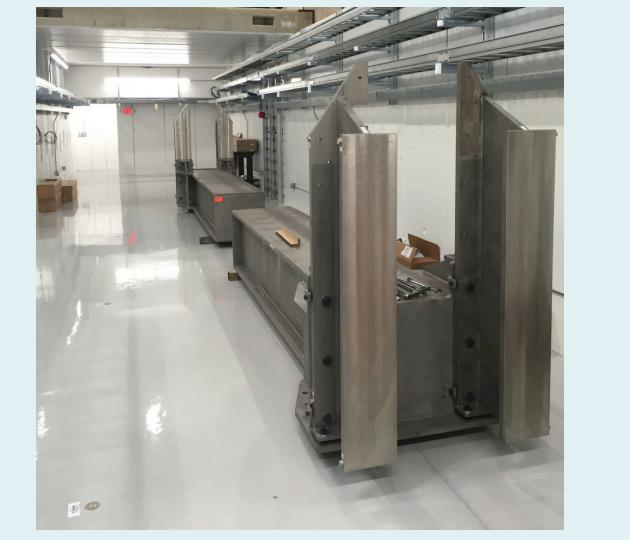
To minimize stray magnetic fields, the cryomodule support girders and hardware within them are fabricated from 316L stainless steel. Each girder bears half of the cryomodule weight, 8,130 lbf.
