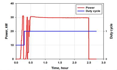
Typical testing procedure: time vs. power and duty cycle.
