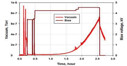
Typical testing procedure: time vs. vacuum and bias voltage.
