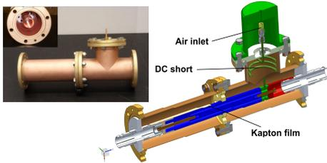
To suppress multipactor in the coupler, high voltage (HV) bias is used. To isolate the coupler input and protect the RF amplifier from HV bias, a DC-block is utilized. The structure of the DC-block is shown. Power requirements for the DC-block are similar to coupler power requirements: reliable operation at power level > 20 kW, CW. Two DC-blocks were installed on the test stand and tested simultaneously with two couplers. A HV bias of up to 5 kV was applied during the test.
