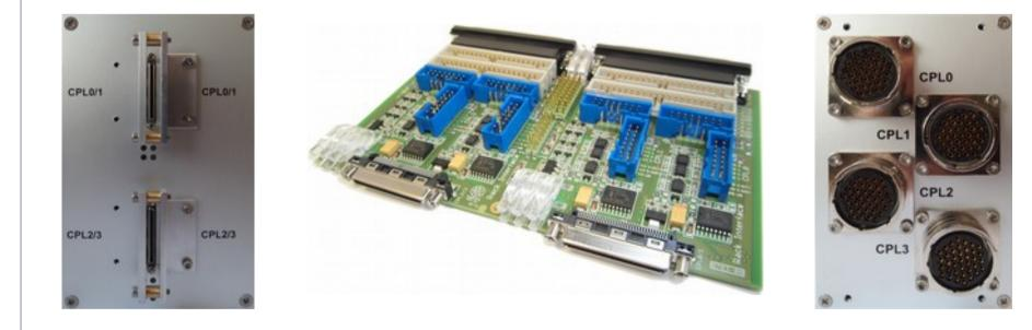
**Coupler-Interface (CPL-IF)** - signal distribution (3\* e-, 1\* Spark, 2\* PT1000) - e- low pass filter and test electronic - unique ID and coupler, module position
