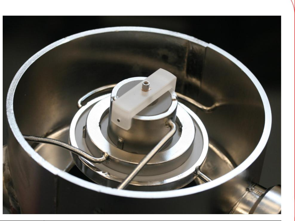
Part of the Sapphire Bridge assembly is a #2-56 NbTi threaded rod, designed to fix the Filter Assembly in place after tuning. These had to be resized, from the original 0.6 inches to 1.01 inches in length.
