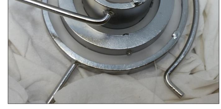
The Filter Assembly is a capacitor made up of concentric Niobium and sapphire rings. The filter assembly is connected to the Tuna Can by means of 1/8" diameter Inductor Rods. Movement of the Filter Assembly along the Main Inductor is the damper's primary tuning mechanism
