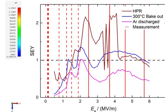
Multipacting simulations indicate soft multipacting barriers in the range between 1.5 MV/m and 5.5 MV/m (depending on surface preparation). Measurements were able to validate the barriers at various gradients.
