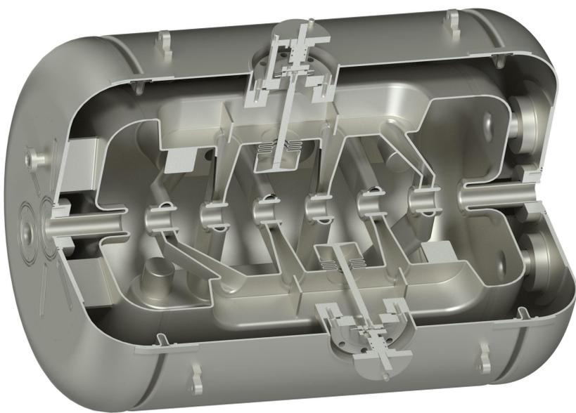
Rendering of the cavity with welded helium vessel.
