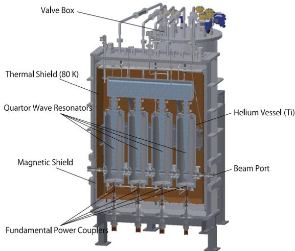
Figure 3: Schematic of a cryomodule for SRILAC.
