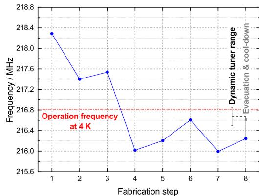
Figure 2: Measured frequency of the sc 217 MHz CH cavity during each fabrication step: (1) temporarily attached end caps with oversize, (2) four static tuners welded in, (3) left end cap welded on, (4) three static tuners welded in, (5) right end cap welded on, (6) 50  $\mu\text{m}$  BCP, (7) two static tuners welded in, (8) 25  $\mu\text{m}$  BCP.
