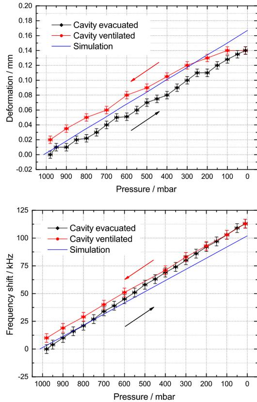
Figure 4: Measured deformation of the cavity wall (top) and related frequency shift (bottom) due to evacuation [6].
