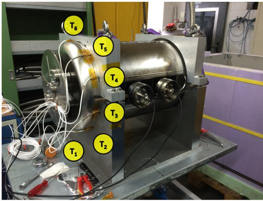
Figure 5: Setup with six temperature sensors to measure the frequency shift during the cool-down with LN<sub>2</sub>.
