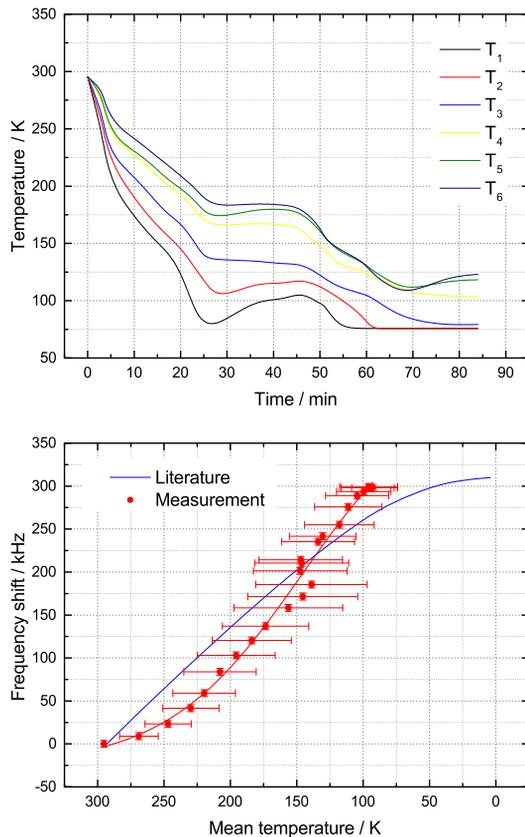
Figure 6: Measured temperature of six probes (top) and related frequency shift (bottom) under cool-down with LN<sub>2</sub>.
