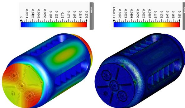
Figure 3: Maximum deformation (left) and von Mises stress (right) of the cavity due to the evacuation process [6].
