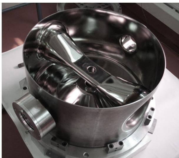
Figure 3: SSR1 resonator being setup to weld the end wall to the shell and spoke assembly.
