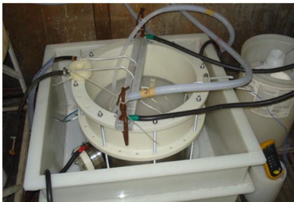
Figure 2: Electro-polishing of the shell sub-assembly at IUAC prior to the EBW of end-walls.
