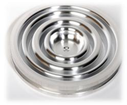
Figure 1: A three-choked 8 GHz test cavity.
