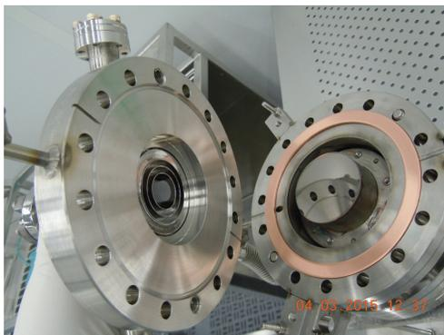
Figure 3: The 100 nm thick  $\text{Nb}_3\text{Sn}$  sample, center right, attached to the calorimeter of SIC before vacuum sealing for the measurements. Sapphire loaded cavity with choke joints is shown on the left.
