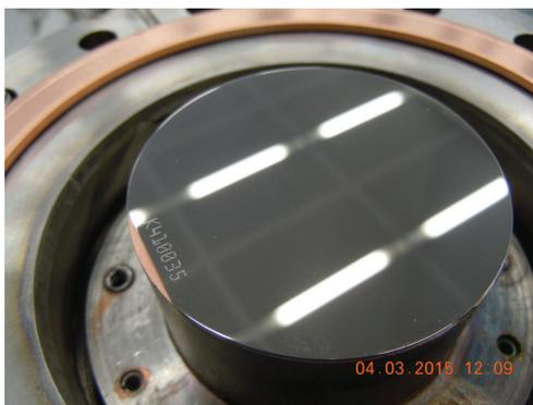
Figure 2: The 100 nm  $\text{Nb}_3\text{Sn}$  film sample attached to SIC calorimeter.
