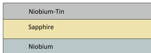
Figure 1: Sketch of the Nb<sub>3</sub>Sn film sample. Nb<sub>3</sub>Sn thickness is 50 nm and 100 nm, correspondingly. Sapphire substrate is 0.3 mm thick and Nb film is ~ 0.2 mm.
