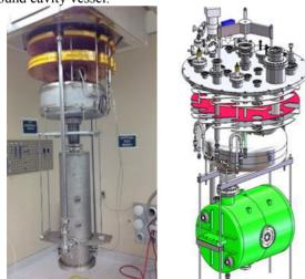
Figure 8: FRIB production insert design.
