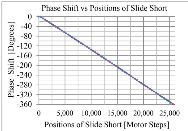
Figure 6: Phase variable range of the phase shifter.
