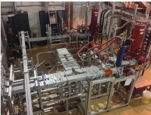
Figure 10: High power rf transmission system of e-Linac phase-I.
