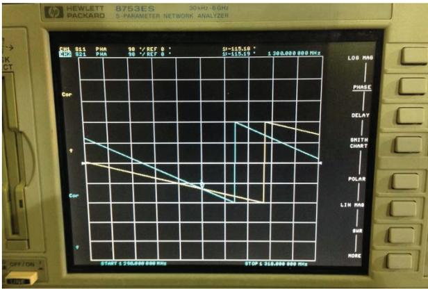
Figure 9: Phase balance between 2 paths of EINJ reached after tuning the phase shifter.
