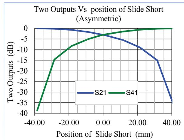
Figure 3: Power division at two output ports in asymmetric structure of the VPD.
