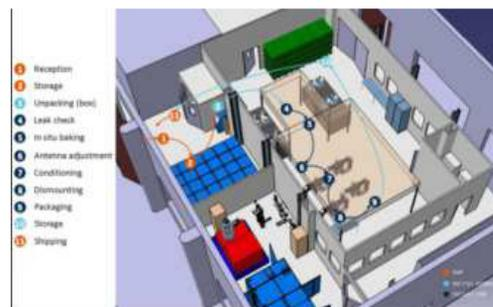
Figure 3: General layout of test bench.
