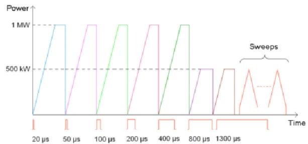
Figure 6: Conditioning sequence applied on couplers.
