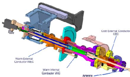
Figure 1: Schematic of XFEL fundamental power coupler.
