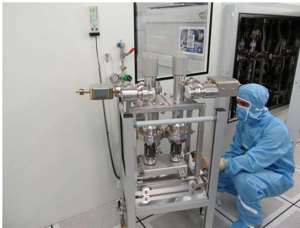
Figure 5: Real implementation of couplers on waveguide box.
