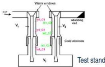
Figure 4: Schematic of FPC on waveguide box.
