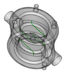
Figure 3: Shell model with an ideal stiffener: zerodisplacement was applied to the interfaces where the stiffener was welded to the cavity central plates (highlighted in green).
