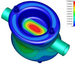
Figure 5: Cavity wall deformation due to radiation pressure at nominal deflecting voltage of 3.34 MV (CST simulation).
