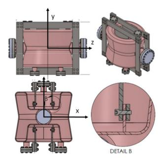
Figure 2: Geometry of the PoP DQWCC with its titanium stiffener.
