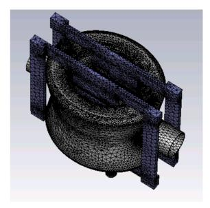
Figure 4: Mesh generated for structural simulation in CST MPhysics solver.
