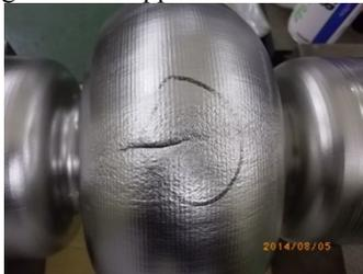
Figure 15: An example of burst during hydro-forming process.
