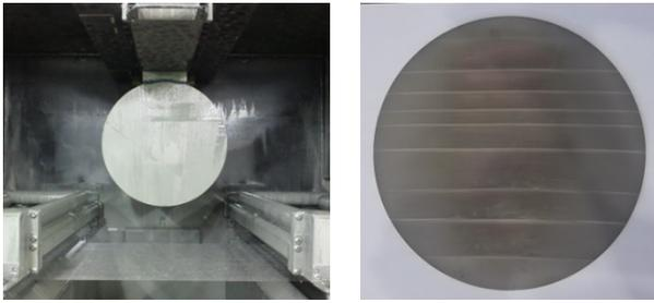
Figure 5: (Left) Slicing large grain Nb ingot by a multi-wire saw and (right) one sliced large grain disk.
