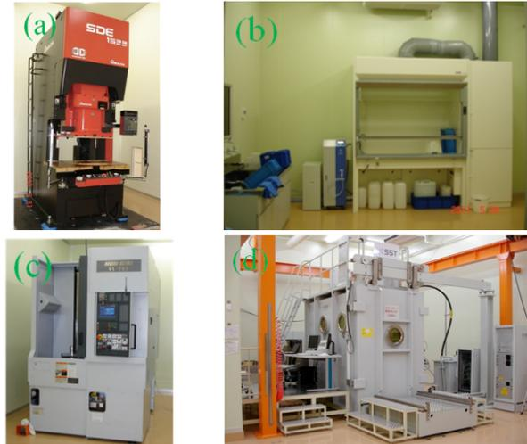
Figure 1: (a) Press machine, (b) CP area, (c) vertical lathe, (d) EBW machine, which are located in KEK-CFF.
