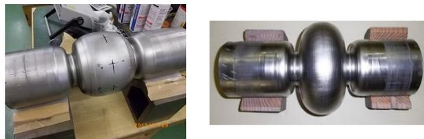
Figure 13: After first stage (left) and second stage (right) of hydro-forming.
