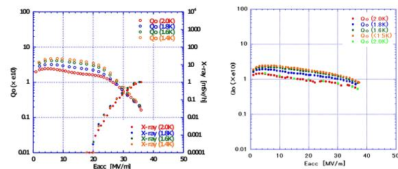
Figure 18: Vertical test results for the W-1 cavity (left) and the U-4 cavity (right).
