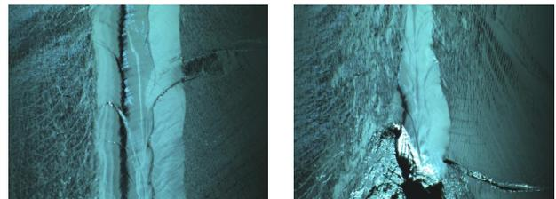
Figure 8: Stable (left) and unstable (right) welding beads for the R-1 cavity.
