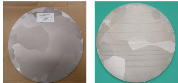
Figure 4: Large grain Nb disk from Tokyo-Denkai (left) and sliced large grain Nb disk from CBMM Nb ingot.
