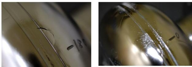
Figure 9: Cracks (left) and spattering (right) observed for the R-5 cavity.
