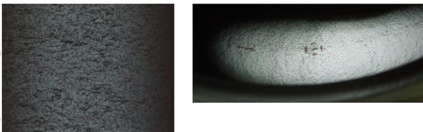
Figure 16: Inner surface of hydro-formed cavity for the W-1 cavity (left) and the U-4 cavity (right) after fabrication.
