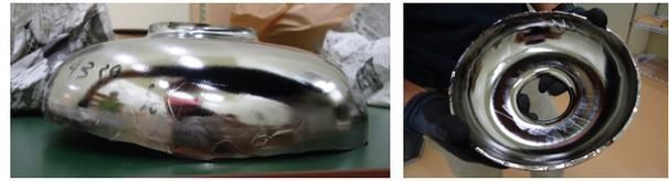
Figure 7: Views of deep-drawn large grain half-cell cavity from side (left) and top (right).
