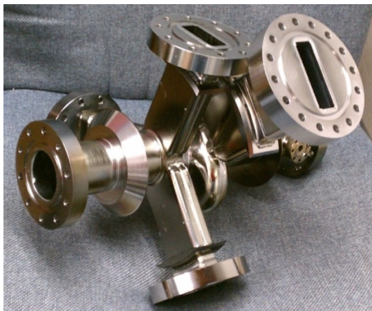
Figure 3: 2.815 GHz TM_{010} crabbing cavity.
