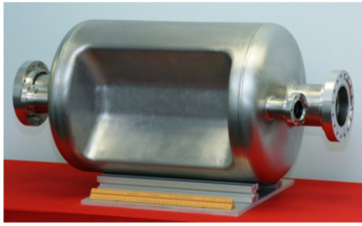
Figure 21: Prof-of-principle 400 MHz rf-dipole cavity.
