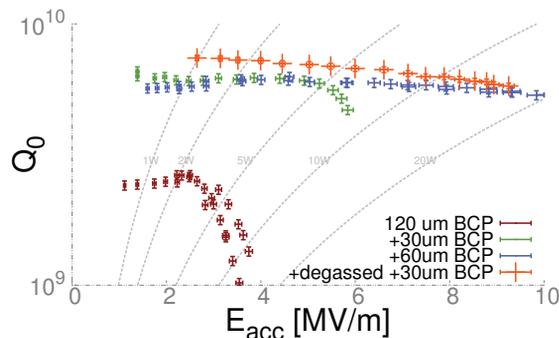
Figure 3: ARIEL3 vertical performance test showed improvements in  $Q_0$  after 800° C degassing.
