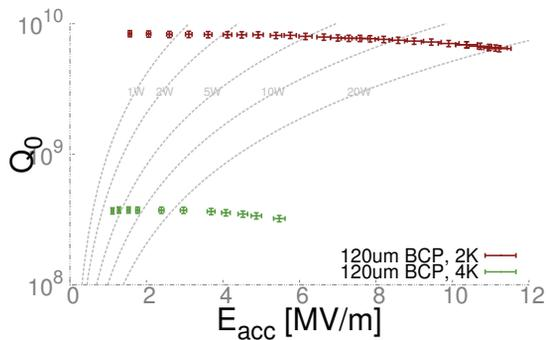
Figure 5: ARIEL4 showed a  $Q_0$  of  $8 \cdot 10^9$  at 2K up to 11 MV/m.
