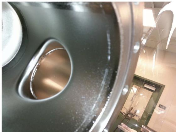
Figure 8: Visible damage on the beam tube cause by the HOM beam line absorbers during assembly.
