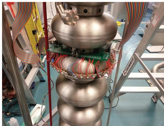
Figure 10: T-mapping test board mounted on a nine-cell cavity ready for testing.
