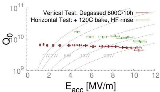
Figure 9: A 120° C bake and HF rinse increased the performance compared to the last vertical test.
