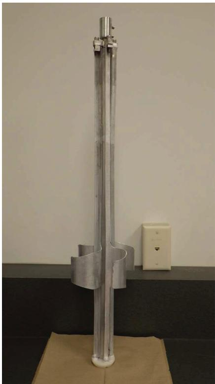
Figure 12: Cathode design of the TRIUMF vertical EP system nick named *D'Sonoqua*.
