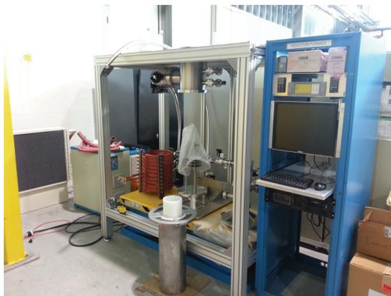
Figure 13: Assembly of the induction furnace for high T degassing.
