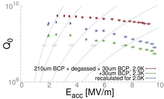
Figure 4: 2.3 K measurements of ARIEL3 showed a decent performance up to 9 MV/m with a moderate slope.
