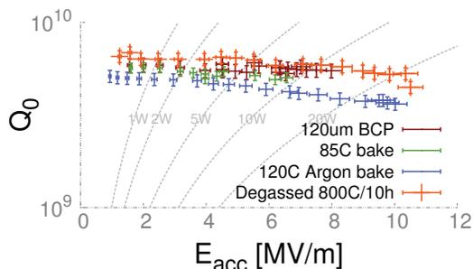
Figure 2: ARIEL2 vertical performance test showed improvements in  $Q_0$  after 800° C degassing.
