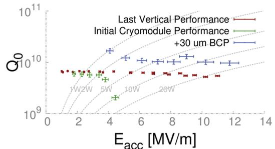
Figure 7: After strong field emissions were found in the cryomodule, a 30  $\mu\text{m}$  etch increased the performance to  $1 \cdot 10^{10}$  up to 11 MV/m.
