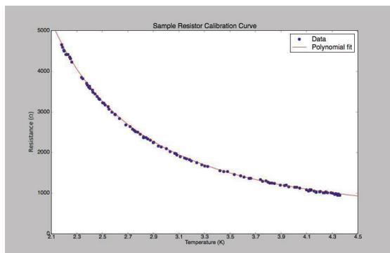
Figure 11: Calibration curve of one of the resistors.
