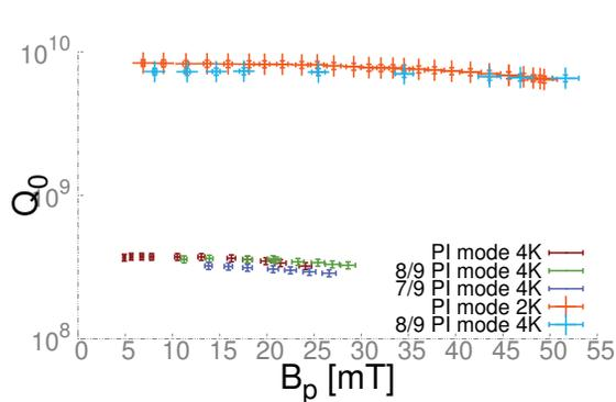
Figure 6: The 7/9 and 8/9 $\pi$  modes showed no difference in  $Q_0$  up to the measured peak surface fields.
