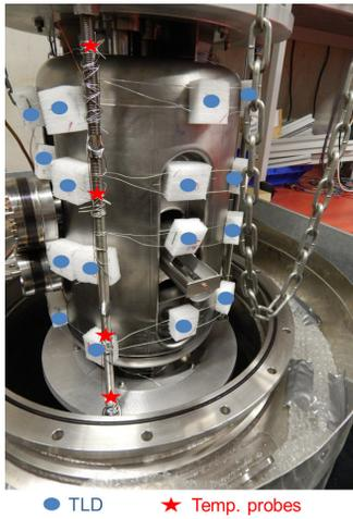
Figure 3: Setup of the cavity with TLDs and temperature probes.
