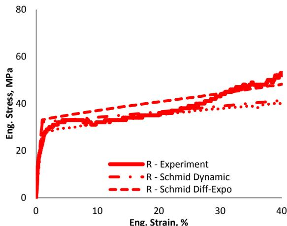
Figure 4: Sample R was used to calibrate the Differential-Exponential model, simultaneously with sample P. This figure also shows the predictions of the Dynamic hardening and the non-Schmid models for sample T.
