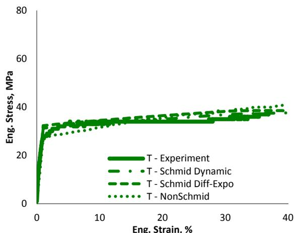
Figure 3: Sample T was used to calibrate the Dynamic hardening and the non-Schmid models, simultaneously with sample P. This figure also shows the prediction of the Differential-Exponential model for sample T.
