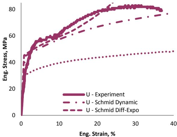
Figure 7: Comparing predictions of the models with the experiment of U. Prediction of the Dynamic hardening model is close to the experiment. The non-Schmid model fail for this sample. The Differential-Exponential model predicts a two-stage behavior for this sample.
