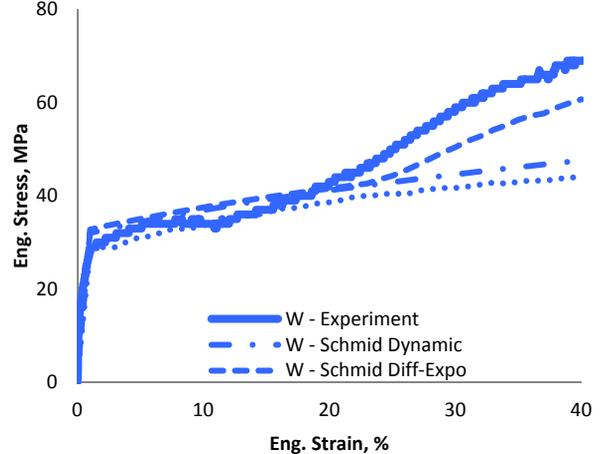
Figure 9: Comparing predictions of the models with the experiment of W. Predictions of the Dynamic hardening and non-Schmid models are close. The Differential-Exponential model predicts a two-stage behavior for this sample.
