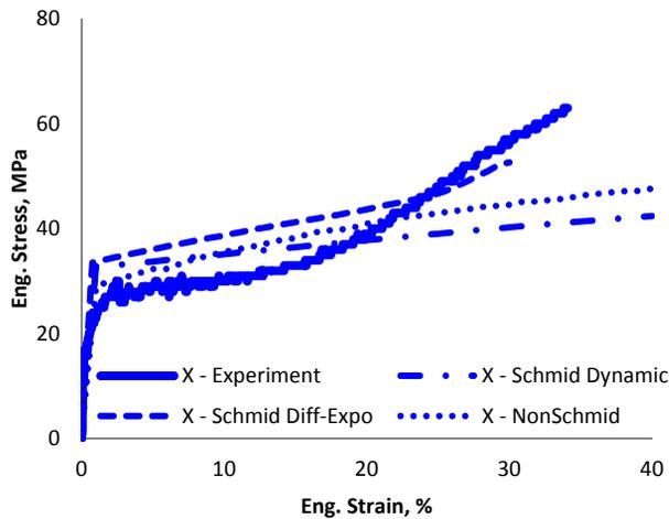
Figure 10: Comparing predictions of the models with the experiment of X. Predictions of the Dynamic hardening and non-Schmid models are close. The Differential-Exponential model predicts a two-stage behavior for this sample.
