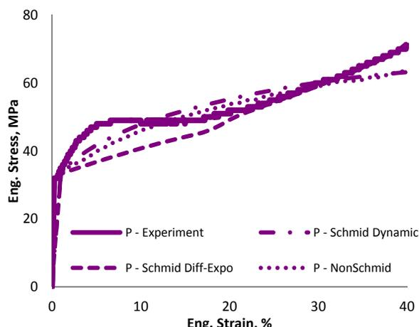
Figure 2: Sample P was used to calibrate all models. Each model was simultaneously calibrated to two experiments. The Dynamic hardening and the non-Schmid models were calibrated with P and T and the Differential-Exponential model was calibrated with P and R.
