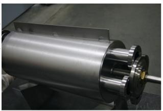
Figure 7: Outer conductor assembled and fitted for the final welding.
