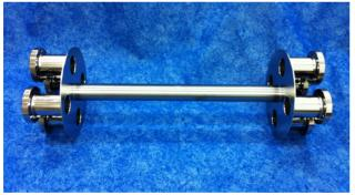
Figure 6: Inner conductor subassembly.
