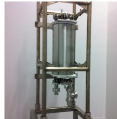
Figure 8: Prepared cavity for a cryogenic test in the clean room.
