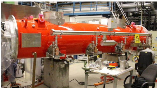
Figure 11: The 3.9 GHz harmonic module during its final preparation stages before installation in the E-XFEL injector tunnel.
