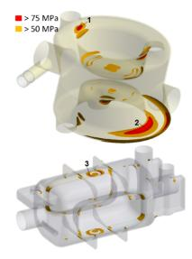
Figure 8: Equivalent stress on cavities - DQW (top) and RFD (bottom).
