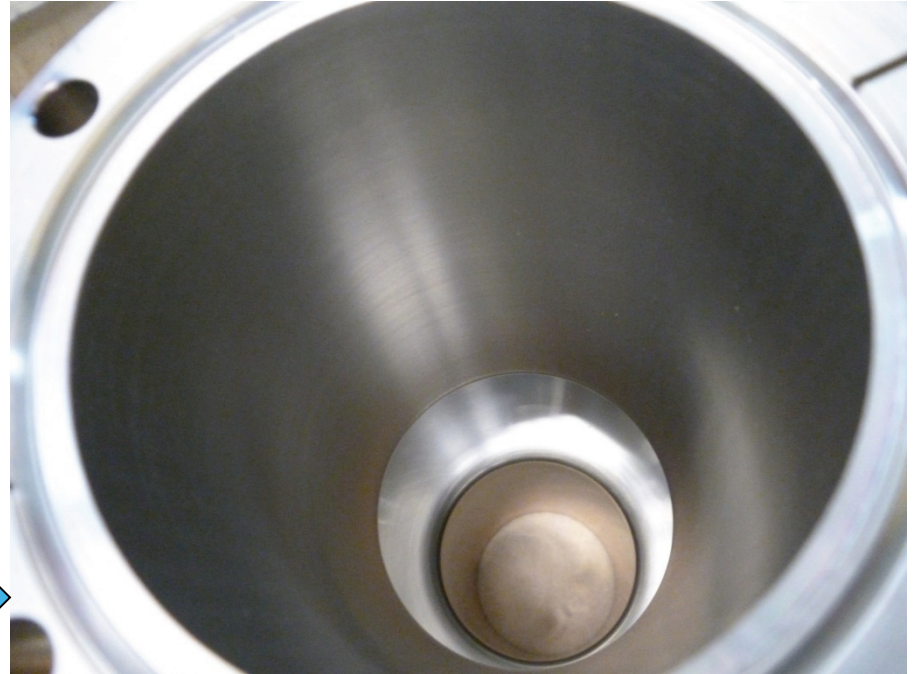
Nb Coating 2 \mu\text{m} Iris / 5 \mu\text{m} beamtubes 350 °C
