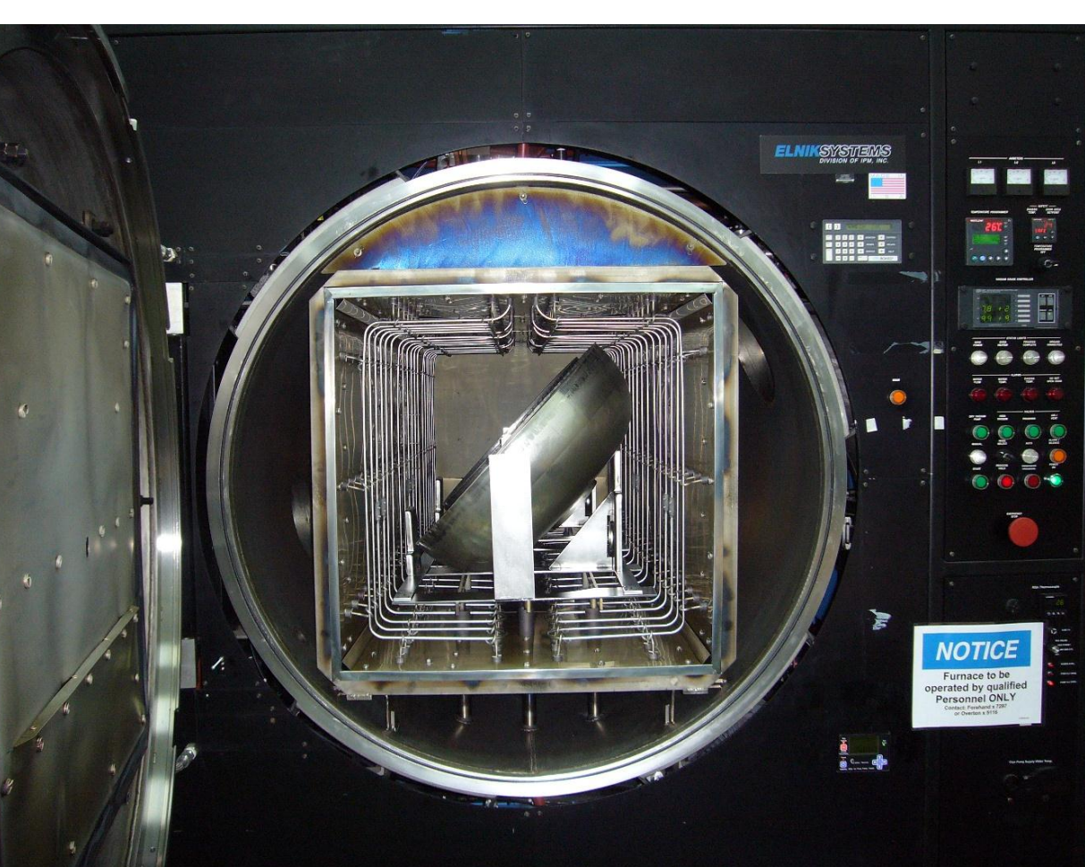
Half cells had to be in an angle during 600C x 10hr annealing
