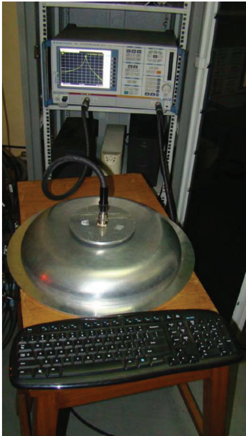
RF Test on Half Cell using VNA
