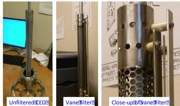
Figure 13: CED electrode configurations: unfiltered (left); vane filtered (middle); expanded view of vane filter (right).
