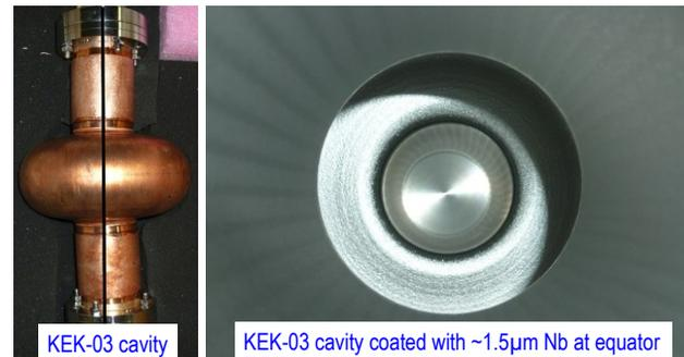
Figure 7: KEK-03 cavity (left) and interior image after coating (right).
