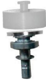
Figure 2: SC Nb sample on holder with protection cap.
