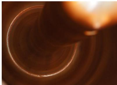
Figure 4: Circular electron beam weld on RF surface.
