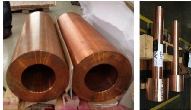
Figure 2: Rough copper forgings for the outer conductors (left) and inner conductors (right).
