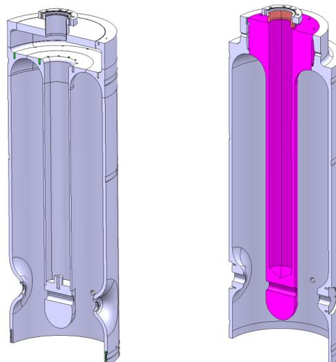
Figure 1: HIE-ISOLDE high-beta copper substrates: left) rolled and welded prototype; right) bulk machined prototype (inner conductor shown in magenta).
