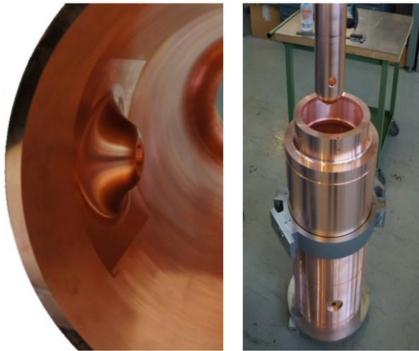
Figure 3: left) detail of beam ports finish; right) Inner and outer conductors being assembled by shrink fit.
