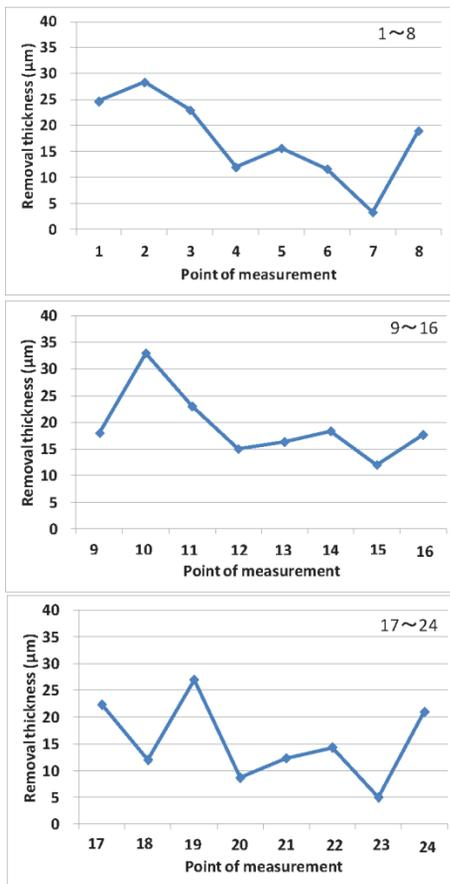
Figure 13: Removal thickness by the third VEP experiment at 24 points on the single-cell cavity. Upper: point 1 – 8. Middle: point 9 – 16. Lower: point 17 – 24. For each point, we measured the thickness three times and took the average before and after the third VEP, and the difference is plotted as the removal thickness.
