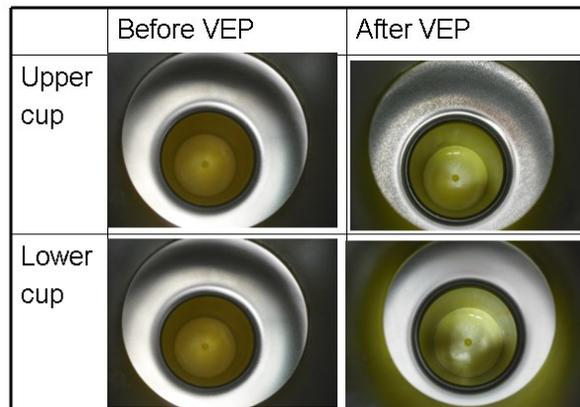
Figure 6: Pictures of inner-surface of cavity before and after the first VEP experiment.
