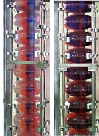
Figure 3: Pictures of experiments in the flow rate of 12 L/min. and in the direction of upward flow. Left-hand side: i-cathode condition of retracted wings without rotation. Colored water has dense distribution and flow near the cathode rod. Right-hand: i-cathode condition of unfolded wings with rotation. The colored water has uniform distribution and flow in the cavity.
