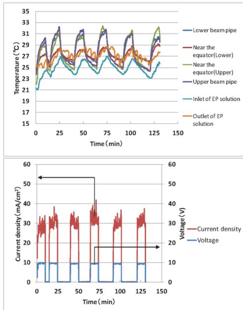
Figure 7: Upper: the plot of temperature vs. time. Lower: the plot of voltage and electric-current density vs. time in the second VEP experiment.
