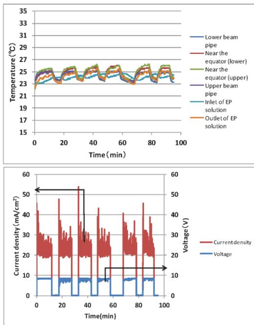
Figure 10: Upper: the plot of temperature vs. time. Lower: the plot of voltage and electric-current density vs. time in the third VEP experiment.
