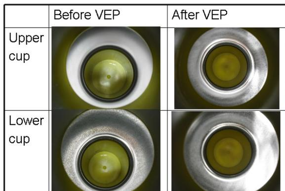
Figure 8: Pictures of inner-surface of cavity before and after the second VEP experiment.
