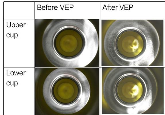
Figure 11: Pictures of inner-surface of cavity before and after the third VEP experiment.
