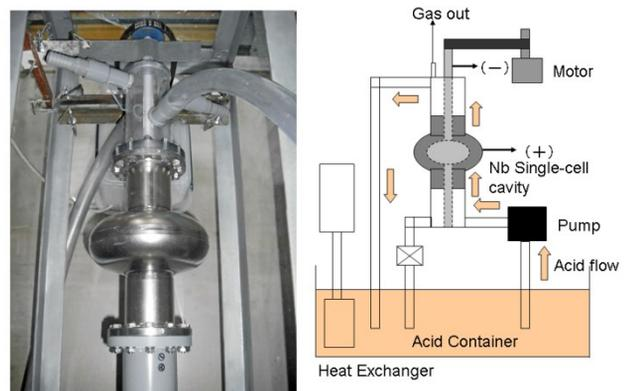
Figure 4: Picture (left-hand side) and schematic view (right-hand side) of setup for the first VEP experiment.
