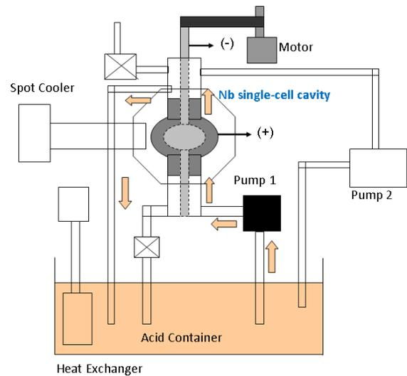
Figure 9: Schematic view of setup for the third VEP experiment.
