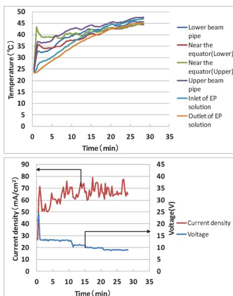
Figure 5: Upper: the plot of temperature vs. time. Lower: the plot of voltage and electric-current density vs. time in the first VEP experiment.
