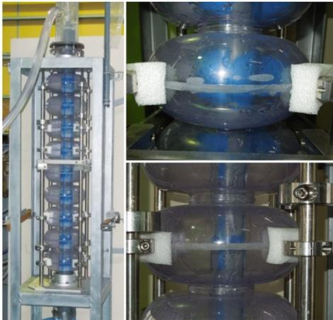
Figure 2: Left-hand side: pictures of setup with a plastic mock-up of 9-cell cavity to see the colored water flow. Right-hand side, upper: wings are unfolded and the cathode rod was rotated. Right-hand side, lower: wings are retracted.
