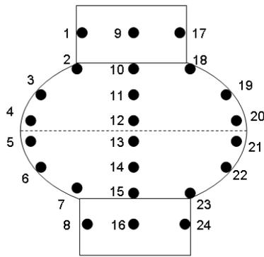
Figure 12: Locations of measured point on the single-cell cavity for the thickness measurements before and after the third VEP experiment.
