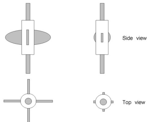
Figure 1: Schematic view of i-cathode “Ninja”<sup>®</sup> for a single-cell cavity. Left-hand side: unfolded status. Right-hand side: retracted/folded status.
