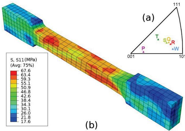
Figure 1(a): The tensile axis of samples used in this study. (b): Simulated deformation of W orientation with the Dynamic hardening model.
