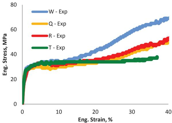
Figure 9: Comparison of tensile experiments of four annealed samples.
