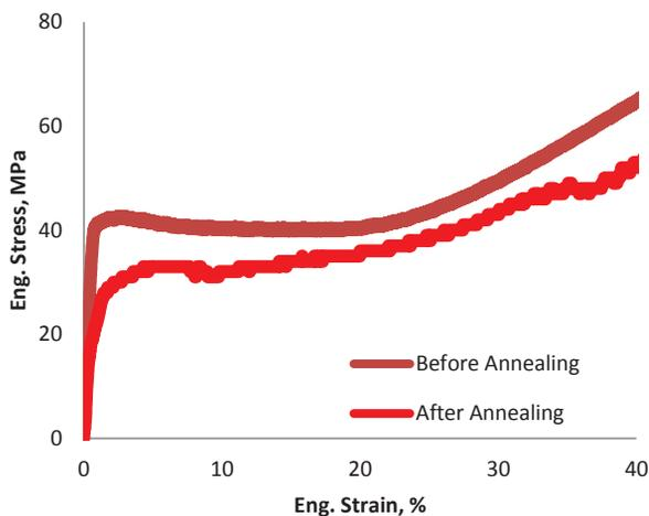
Figure 3: The effect of annealing on the engineering stress-strain response of an Nb tensile sample (Material Orientation R).
