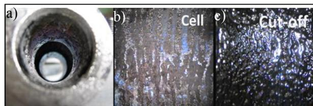
Figure 7: Vertical electropolishing of cavity: a) top part; b) cell; c) cut-off.
