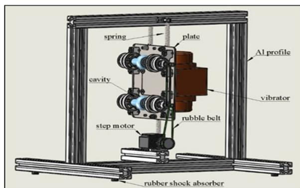
Figure 2: Schematic drawing of the vibrating system.
