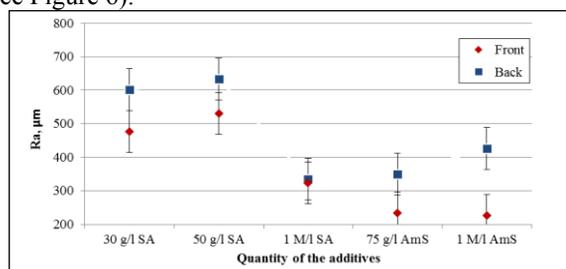
Figure 6: The dependence of surface roughness on the additives concentration.
