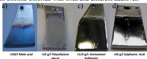
Figure 5: Samples treated in Choline Chloride and Urea (ratio 1:4) with: a) 1M/l Malic Acid; b) 10 g/l Polyethylene glycol; c) 1 M/l Ammonium Sulfamate; d) 50g/l Sulphamic Acid.
