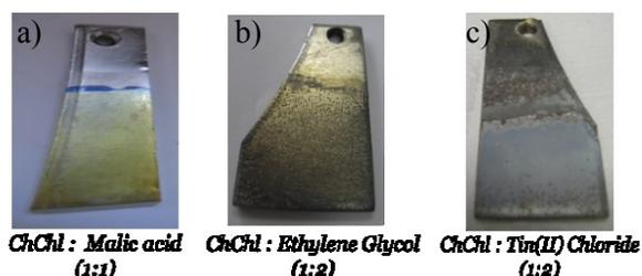
Figure 4: Samples treated in new Ionic liquids: a) 1 ChChl: 1 Malic acid; b) 1 ChChl: 2 Ethylene Glycol; c) 1 ChChl: 2 Tin (II) Chloride.
