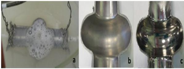
Figure 9: Horizontal electropolishing of half cavity: a) during the process; b) before treatment; c) after treatment.
