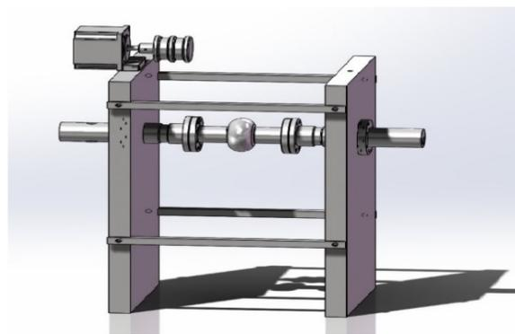
Figure 1: System for horizontal electropolishing.
