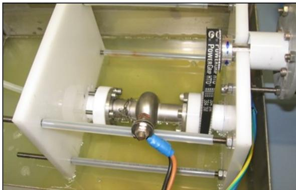
Figure 10: The new system for the electropolishing half of cavity.
