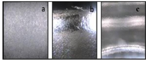
Figure 11: Cell before and after Electrochemical polishing in New system: a) before, b) and c) after.
