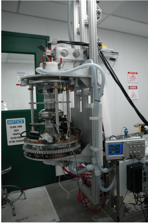
Figure 3: Vertical bipolar EP configuration.
