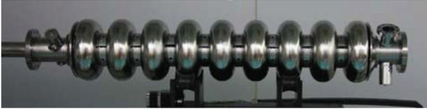
Figure 1: large grain 9-cell superconducting cavity (PKU4).
