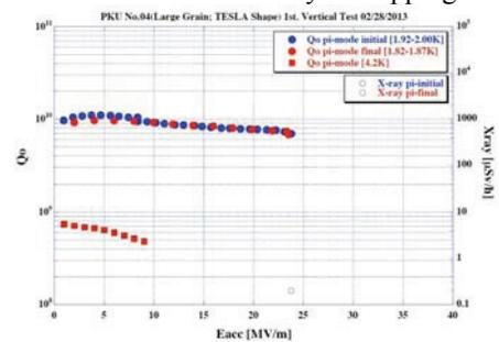
Figure 3: the first vertical test result of PKU4.
