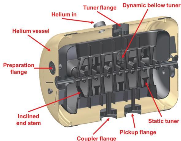
Figure 2: The sc 217 MHz CH cavity.
