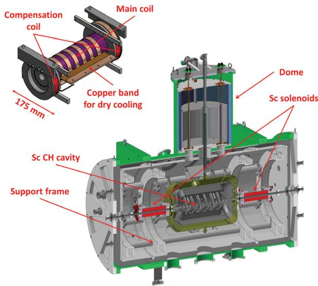
Figure 5: Final layout of the horizontal cryomodule and of the sc 9.6 T solenoid for the cw demonstrator at GSI.
