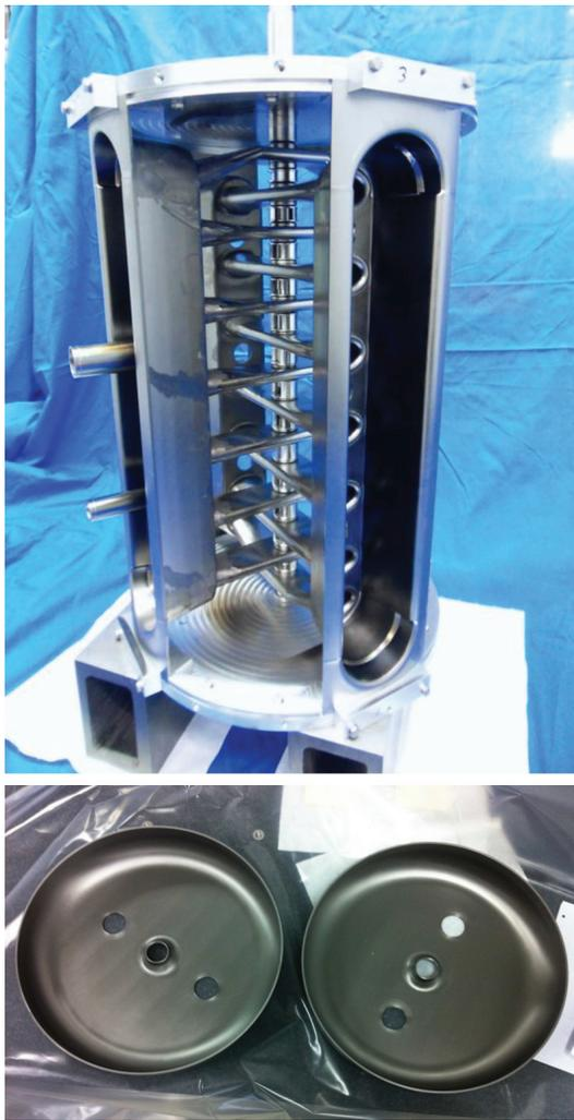
Figure 3: Fabrication status of the cavity: Assembly of the cavity components (top) and end caps after hydro forming (bottom).
