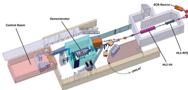
Figure 1: Future test set-up at GSI. The existing HLI will be used as an injector for the cw demonstrator.
