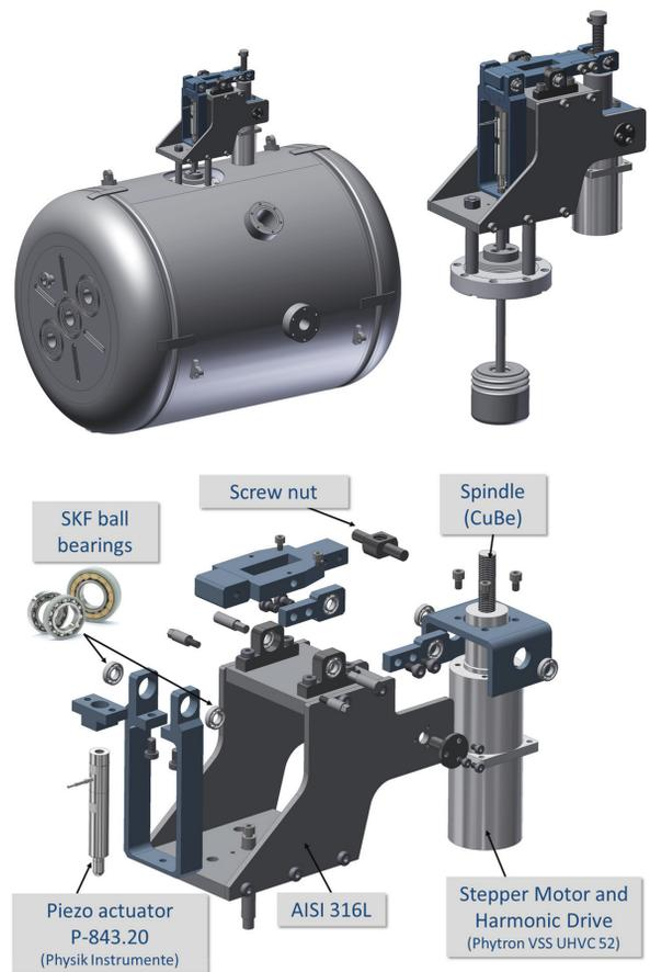
Figure 4: Tuner drive mounted to the helium vessel of a sc CH cavity and frequency tuning system including dynamic bellow tuner (top), exploded view drawing of all single components of the tuner drive (bottom).
