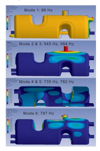
Figure 6: Cavity deformation due to the first six mechanical modes.
