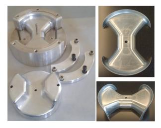
Figure 8: Half-scale spoke die (left) and aluminum spoke halves pressed with the die.
