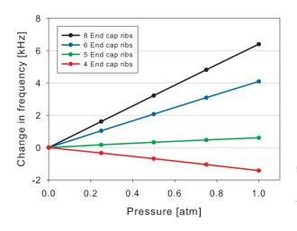
Figure 4: Change in frequency (from 500 MHz) for varying numbers of end cap stiffening ribs. Here, 1 atm external pressure was applied equally to the entire cavity.
