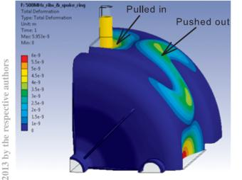
Figure 5: Cavity deformation due to LFD enhanced by a factor of  $4.1 \times 10^6$ .
