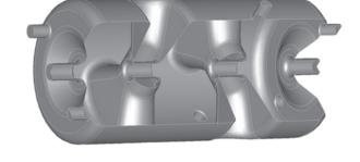
Figure 1: 500 MHz,  $\beta_0 = 1$  double-spoke cavity concept.
