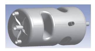
Figure 3: 3 mm cavity with 4 mm thick spokes and end cap stiffening ribs.
