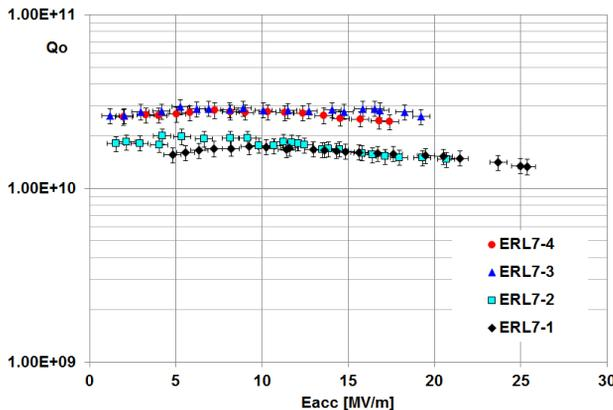
Figure 9: Q curves for the 4 ERL cavities tested so far. All data were taken at 1.8 K.
