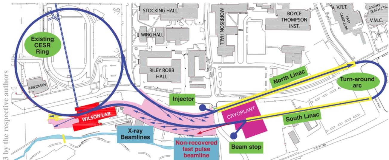
Figure 1: The proposed Cornell ERL, transforming the existing CESR storage ring into a high brightness coherent X-ray source.
