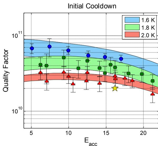
Figure 2:  $Q$  versus  $E$  of the first ERL cavity, mounted inside the HTC cryomodule, fully equipped with power coupler and HOM absorber.
