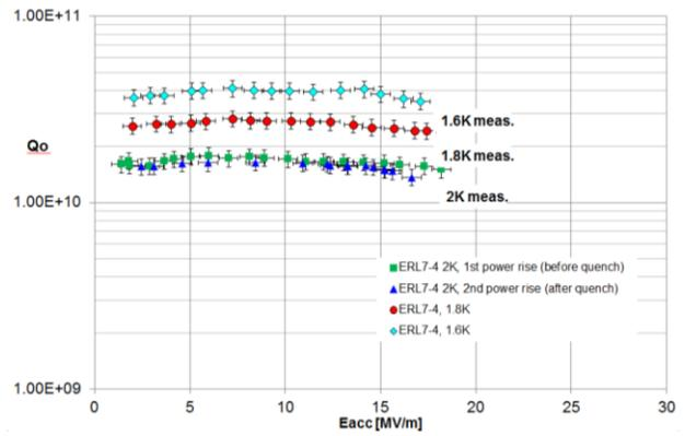
Figure 7: Q-curves for the latest produced ERL cavity (ERL7-4), achieving  $2.5 \cdot 10^{10}$  at 16 MV/m and 1.8 K.
