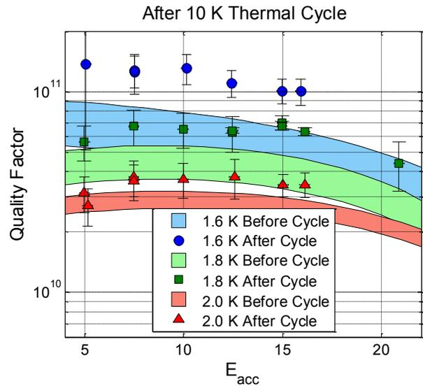
Figure 3:  $Q$  versus  $E$  for the same cavity after going through a 10 K thermal cycle. A significant  $Q$  increase could be measured.
