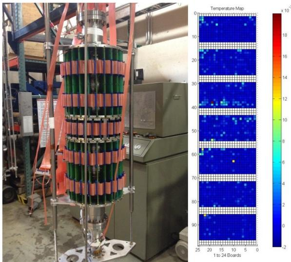
Figure 8: The Cornell T-map system as it is installed around an ERL cavity (left) and the heating map we got on ERL7-4 (17 MV/m, 2K).
