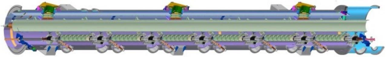
Figure 5: CAD model of the cryomodule prototype (MLC). It will house 6 ERL type cavities. More details are given in the text.
