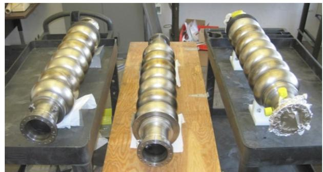
Figure 6: Three ERL cavities built at Cornell to be installed into the prototype Main Linac Cryomodule (MLC).
