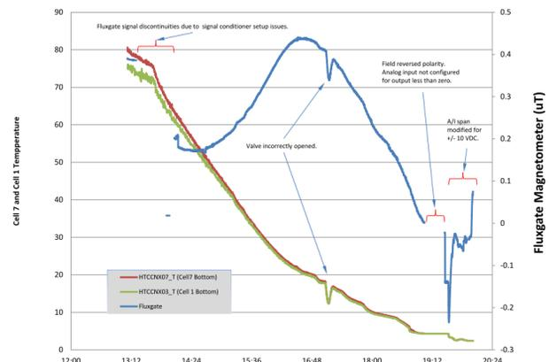
Figure 4: Magnetic field measurement during initial cooldown of the HTC-3. The flux gate sensor was mounted outside the helium tank but inside the second layer of magnetic shielding.
