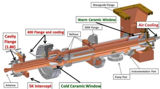
Figure10: RF Power coupler. The coaxial transmission line has two bellows which allow for lateral movement during cool-down.
