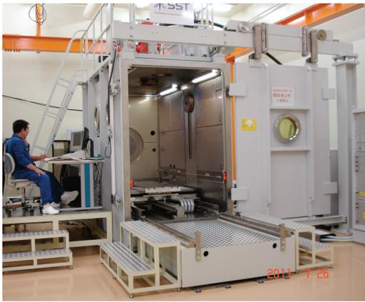
Figure 2: The EBW machine installed in CFF.
