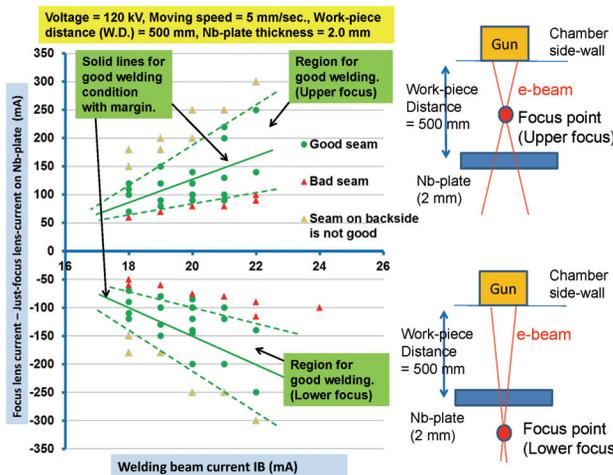
Figure 7: Example of basic welding test.
