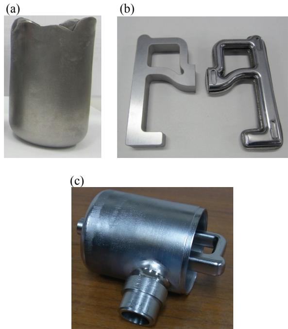
Figure 8: New manufacturing method for HOM coupler, deep drawn niobium cup ( $\phi 48 \times 64$ ) (a), antenna (left; before press forming, right; after press forming) (b) and assembled HOM coupler (c).
