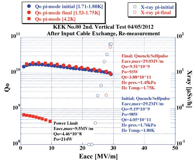
Figure 5: Q-E curve of the vertical test for KEK-0.
