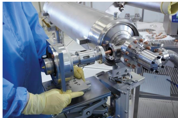
Figure 6: coupler to cavity connection in the clean room with tools (elevator table and coupler holding).
