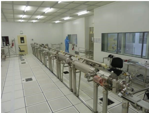
Figure 4: PXFEL2_2 in the ISO4 clean room facility.
