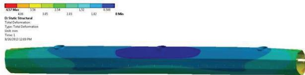
Figure 17: Shield deformation when the temperature gradient reaches the maximum.
