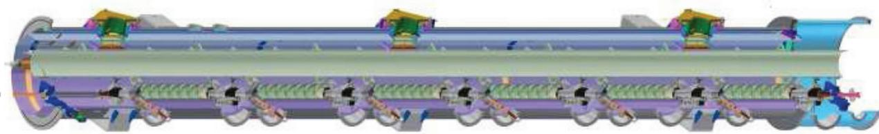
Figure 1: CAD model of the cryomodule prototype.
