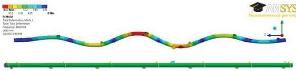
Figure 19: Lowest mechanical eigenmode of 2-phase pipe and the model showing the supports.
