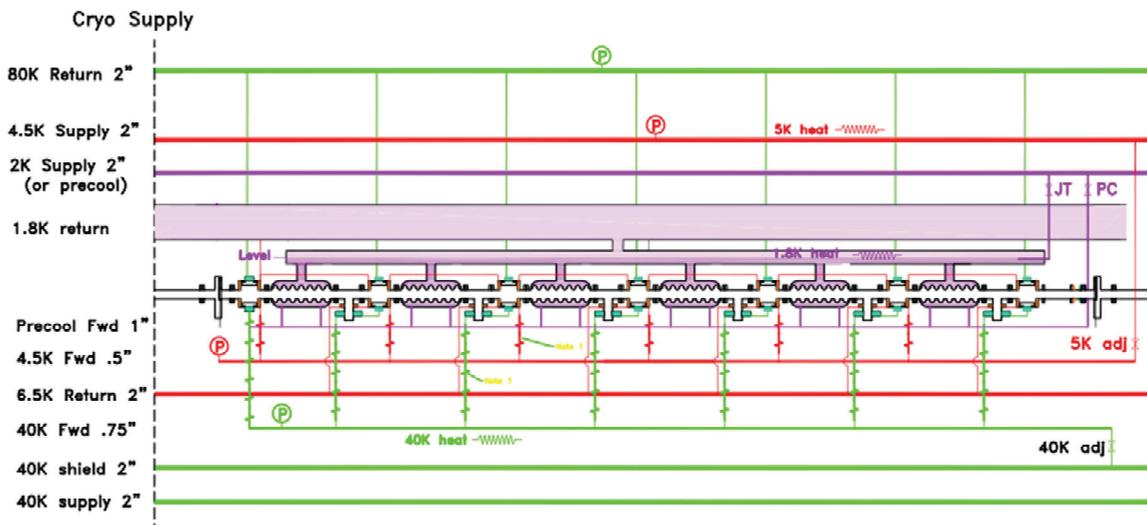
Figure 9: Diagram of the cooling loops in the module.
