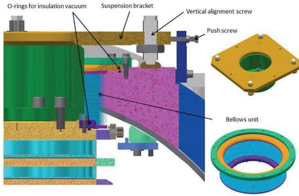
Figure 6: Post alignment components.
