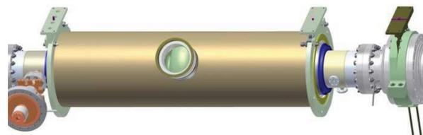
Figure 5: Beam-line support plates with pin/key for alignment.
