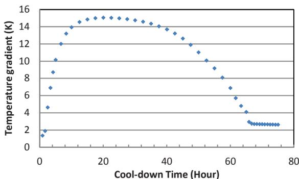
Figure 15: Temperature gradient on 40 K shield as a function of time during cool-down.
