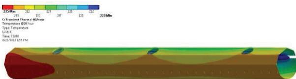
Figure 14: Temperature distribution on the shield at 20 hours after cool-down started.
