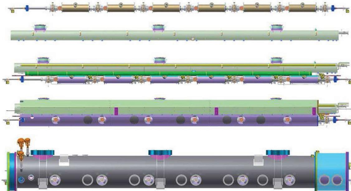
Figure 20: MLC prototype assembly sequence.
