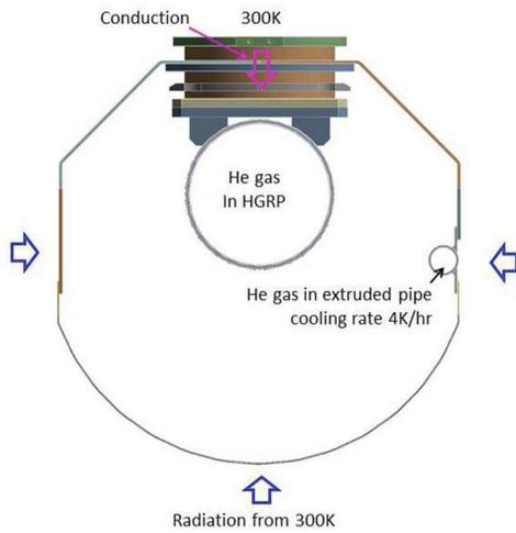
Figure 13: Asymmetric cooling of the 40 K thermal Shields.
