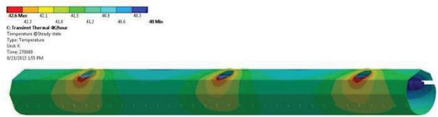
Figure 16: Temperature distribution of the shield at steady state.
