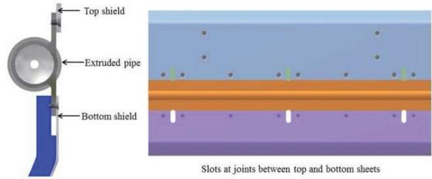
Figure 8: Joints between top and bottom sheets.
