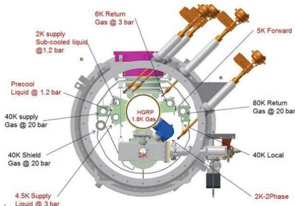
Figure 11: Cross-section of the module.
