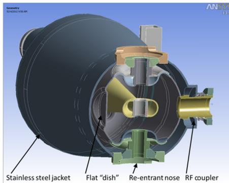
Figure 2: A half cavity model in ANSYS.
