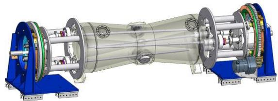
Figure 4: 3D model of the cavity with electropolishing cathodes inserted through two ports at each end.
