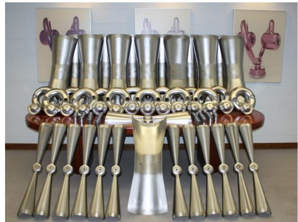
Figure 8: Nb parts for PXIE production cavities.
