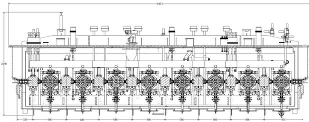
Figure 5: The side cross-section of HWR cryomodule for PXIE.
