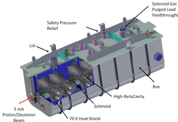
Figure 6: Assembly of the high- $\beta$  cryomodule for SARAF.
