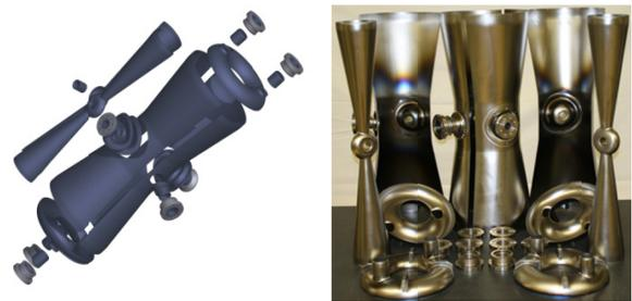
Figure 3: Modelled (left) and actual (right) niobium parts of the cavity.
