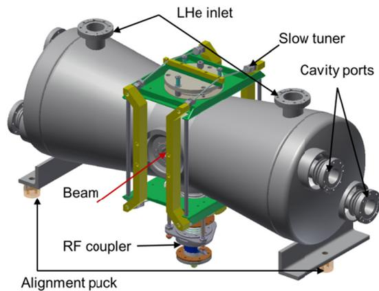
Figure 1: A cavity 3D model in INVENTOR.
