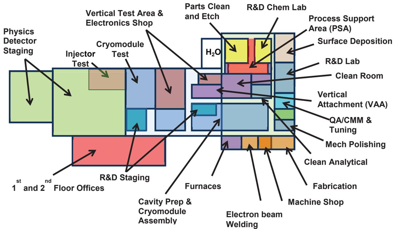
Figure 1: Overview schematic of new Test Lab/TEDF SRF facilities at Jefferson Lab, occupied summer 2013.
