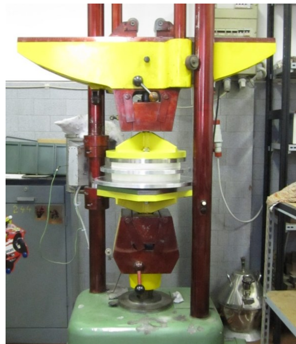
Figure 4: Traction test of a support post.
