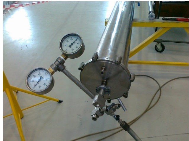
Figure 3: Pressure test of a process pipe.
