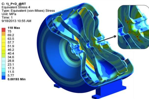
Figure 3 : Von Mises stress distribution in a spoke resonator subject to 2 atmospheres of pressure in the helium space. Values above the yield limit are shown in red.
