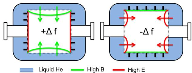
Figure 4 : A schematic view of a resonator subject to an increase in liquid helium pressure. Different stiffening systems produce different deformations. Inward deformations in high B areas (left) or high E areas (right), generate positive or negative frequency shifts respectively.
