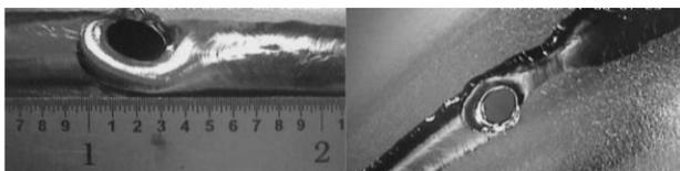
Figure 5 : A typical blow-through viewed from the outside (left) and from the inside of the cavity (right).
