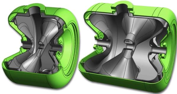
Figure 2 : Sectioned views of SSR1 (left) and SSR2 (right). Niobium components are rendered in gray, steel components are rendered in green. The rounded end-walls in SSR2 require fewer stiffeners than SSR1.
