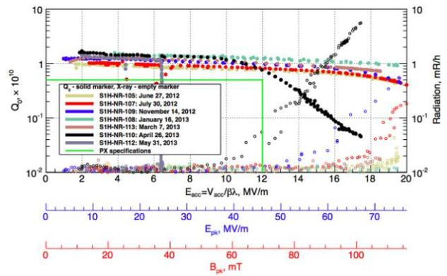
Figure 6 : Summary of the qualification process for SSR1 resonators. All plots refer to testing at 2 K.
