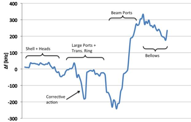
Figure 9 : Plot showing the history of resonant frequency during welding operations. The overall shift was about 250 kHz.
