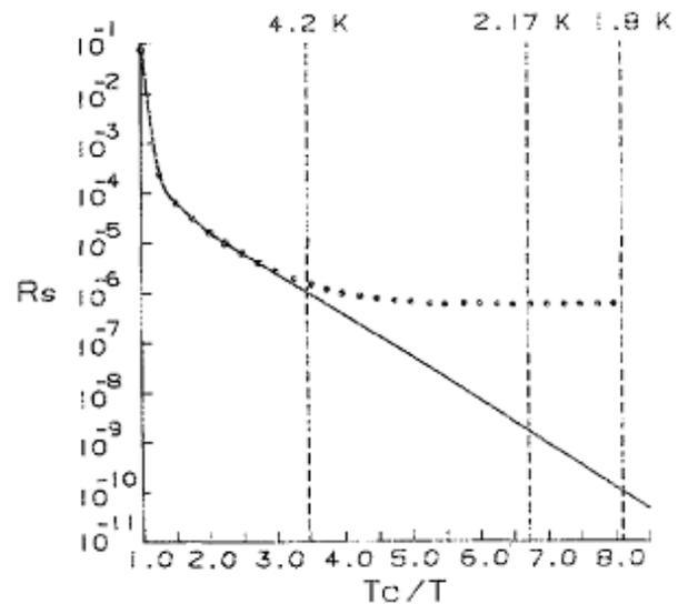
Figure 2:  $R_s$  vs.  $T$  for 4.5 GHz NbN cavity, made by nitridation of a niobium cavity. Note,  $R_s$  of this cavity at 4.2 K, 1.15  $\mu\Omega$ , is lower than that of niobium at this temperature and frequency,  $\approx 2.5 \mu\Omega$ . This NbN cavity, however, had a high residual resistance of about 0.69  $\mu\Omega$ , [9].
