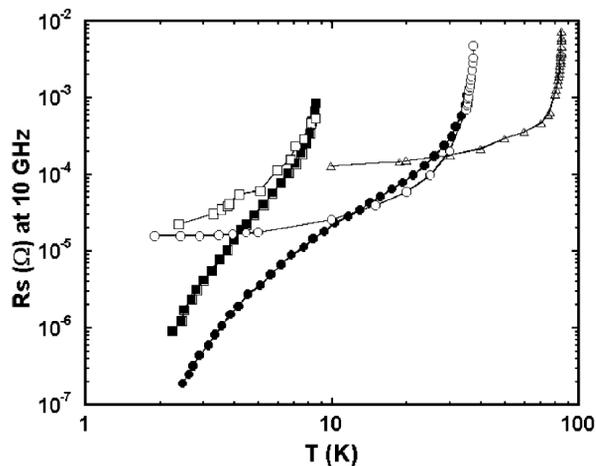
Figure 4:  $R_s$  vs.  $T$  scaled to 10 GHz for  $MgB_2$  films, deposited by the reactive evaporation technique, [13], on sapphire (circles), a YBCO film on LAO (triangles), and for Nb thin films (squares). Filled symbols indicate the parallel plate measurements with external losses subtracted, and open symbols indicate stripline resonator measurements including external losses, [14]. Note that at 4 K the resistance of  $MgB_2$  film is about 5 times lower than that of Nb.
