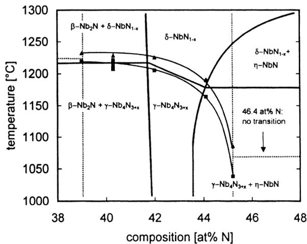
Figure 1: The phase diagram of Nb-N system around the phases of interest for SRF applications,  $\delta$ -phase and  $\gamma$ -phase, from [6].
