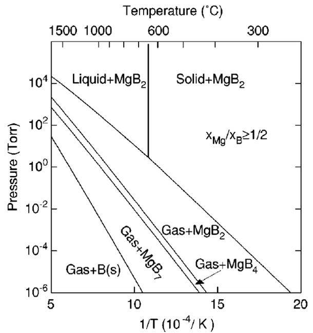
Figure 3: The phase diagram of the Mg-B system from [12].
