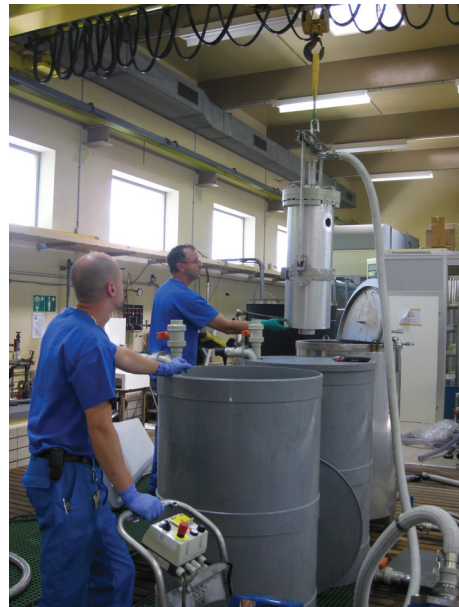
Figure 1: The three tanks in line for the QWR chemical polishing.
