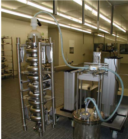
Figure 2: Set up of alcohol cleaning apparatus at DESY
