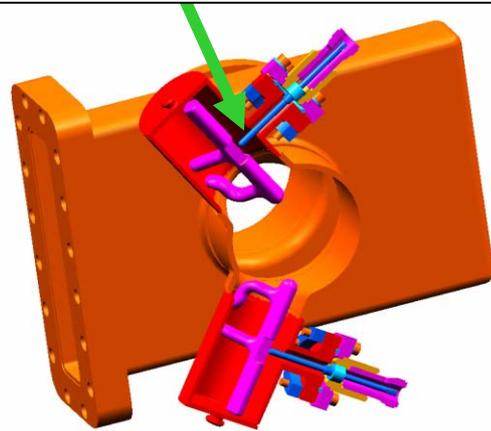
Figure 1. HOM coupler configuration in the CEBAF *Renascence* prototype cavities, locating the critical cooling situation.
