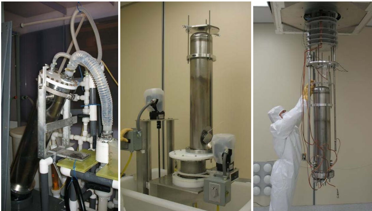
Figure 4. Left to right: etching, rinsing, and assembly of the \beta_m = 0.041 QWR onto the RF test stand.
